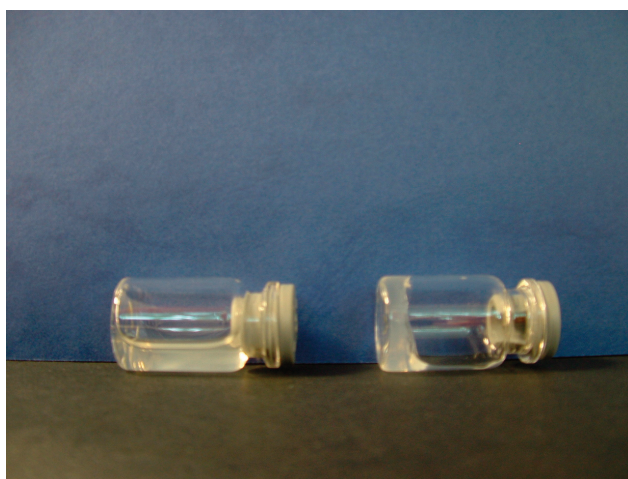
Figure 2. Photograph to show appearance of PecSys™ before (left-hand vial) and after (right-hand vial) exposure to simulated nasal electrolyte solution.
